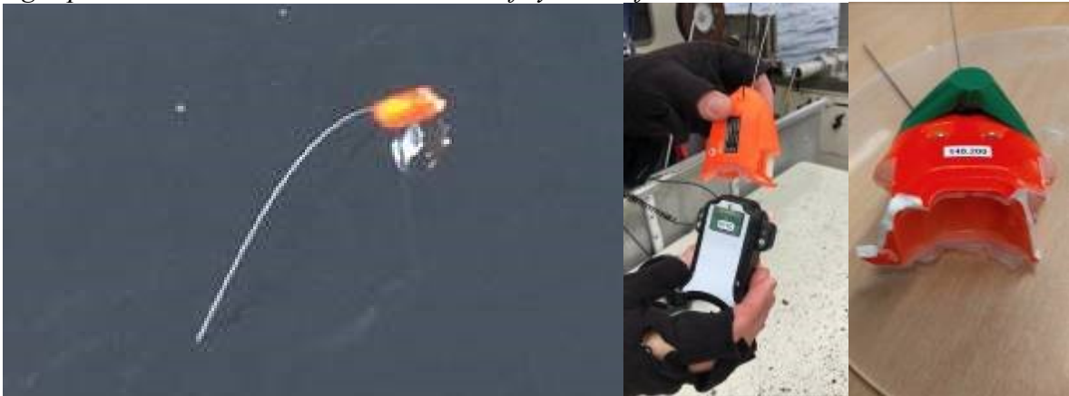
Figure 4C. Left panel shows the Dtag3+ was floating at sea with a broken housing. The right-panel below shows the broken areas of syntactic foam.
